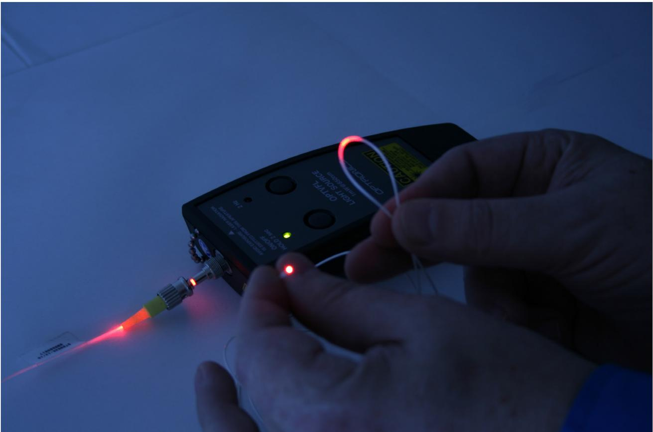
Picture 1: Detecting Macrobending with a VFL
